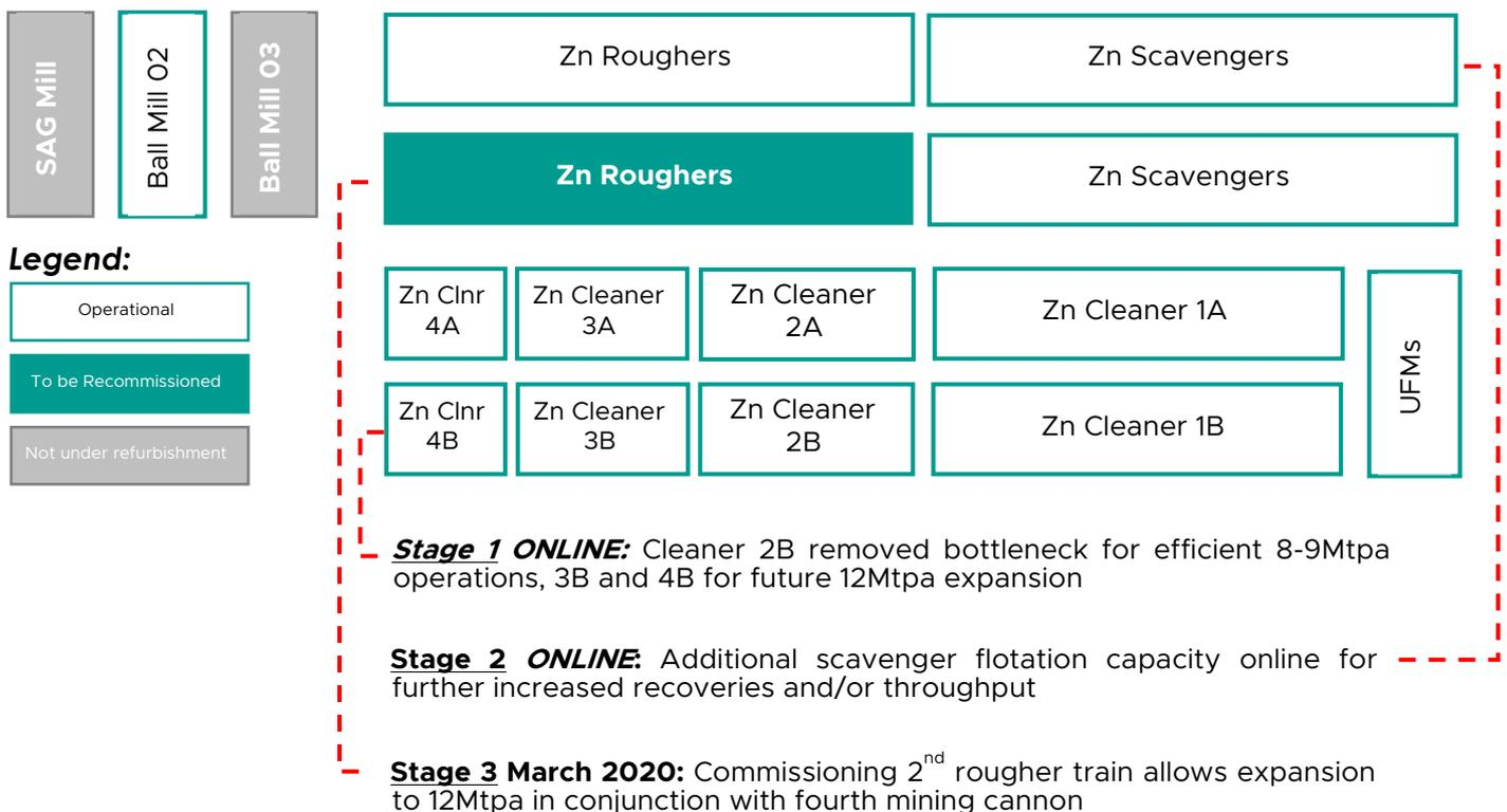
**Figure 4: Simplified plant plan view & scheduled 12Mtpa expansion progress**
