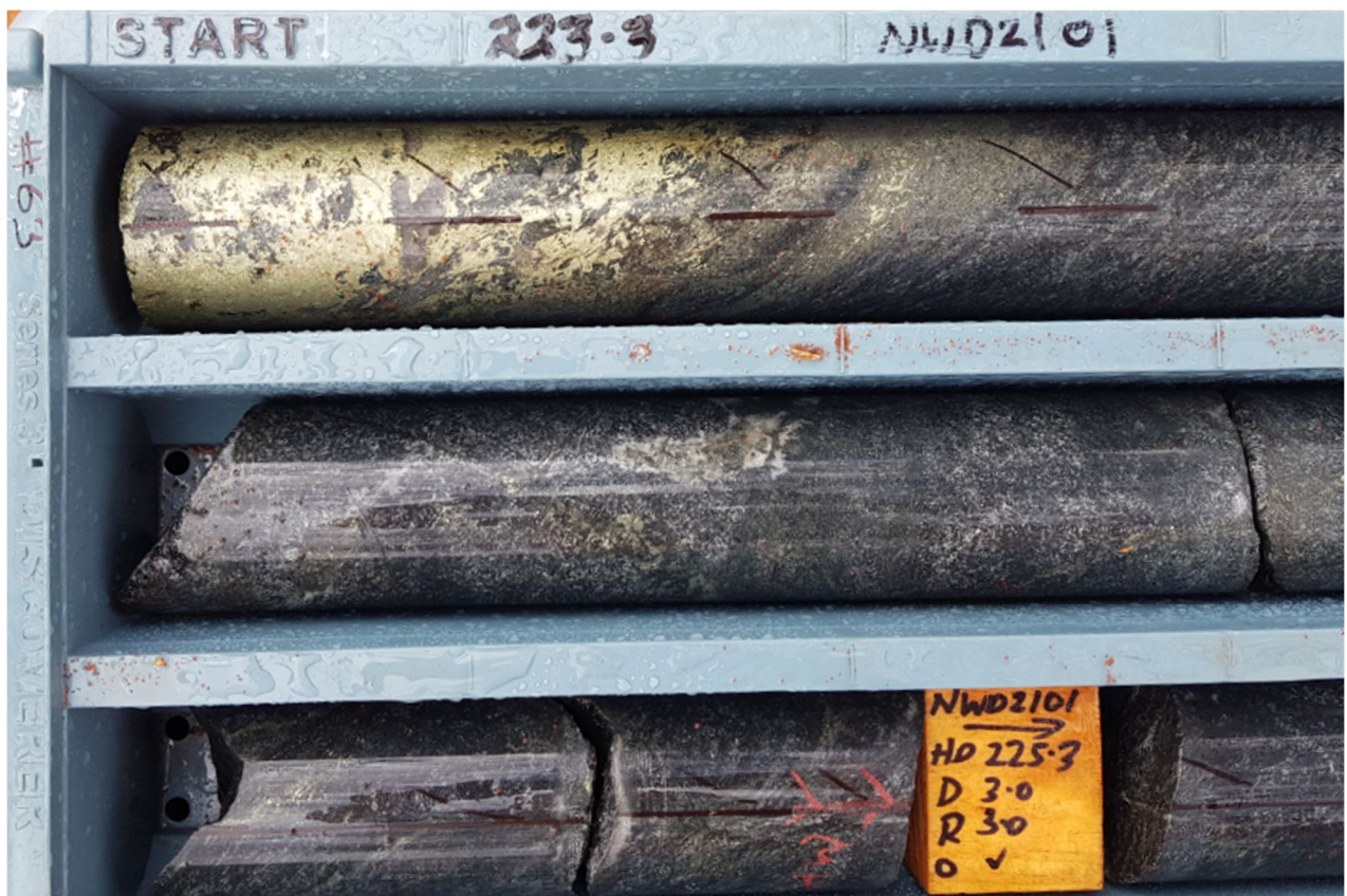
Image 1 | NWD2101 drill core 223.3m to 225.3m downhole showing chalcopyrite copper sulphide mineralisation
